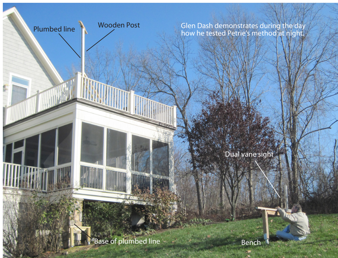
Below: Testing Petrie's method in Pomfret, CT (latitude N 41 degrees, 54 minutes, 7.3 seconds; longitude W 71 degrees, 58 minutes, 13.6 seconds; elevation 182 meters above mean sea level). A wooden pole set up on a second story porch substituted for Petrie's masonry wall. The pole held a plumb line that was fixed at its base. The observer sights a star through the vanes of the sliding sight. Photo by Joan Dash.
